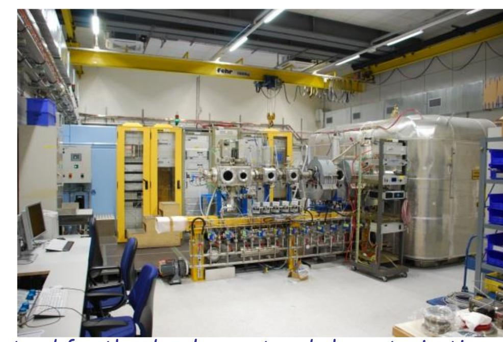
Test stand for the development and characterisation of proton sources for the PSI proton cyclotron.
