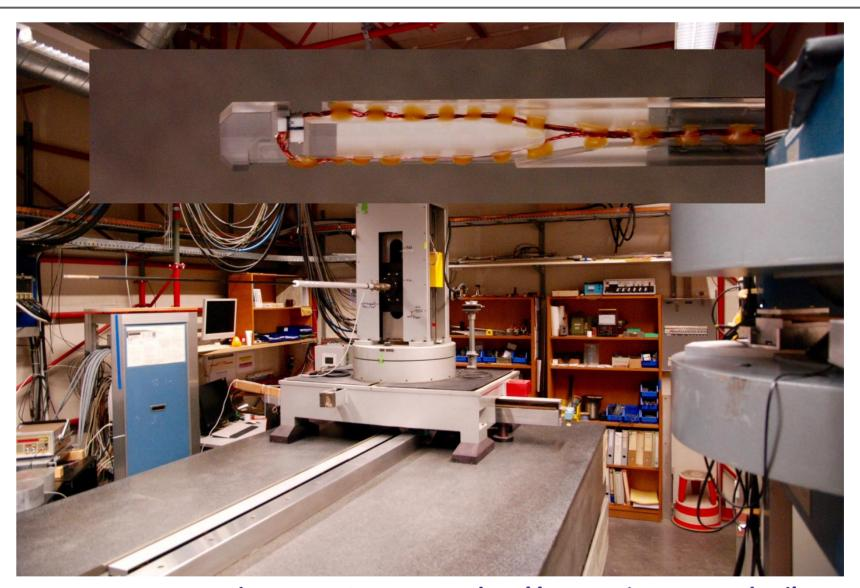
The magnet test stand is a 3-axis hall probe with "sensing" volume of 100x100x100 μm cubed mounted on a long lever arm. The 'inset' shows a close up of the probe.
