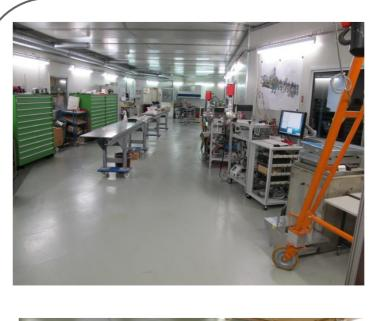
In order to ensure that all accelerator components meet the strict vacuum requirements imposed upon them we have a fully equipped vacuum test laboratory in which vacuum chambers can be qualified before installing them in an accelerator or on a beamline.
