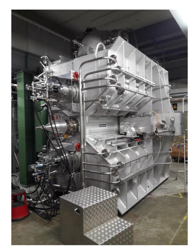
The large 50 MHz resonators for the injector ring and main ring of the high intensity proton accelerator require a test facility to measure their performance and to test low level RF control systems with them. The picture on the right shows one of the new Injector resonators built as part of the HIPA up-grade.
