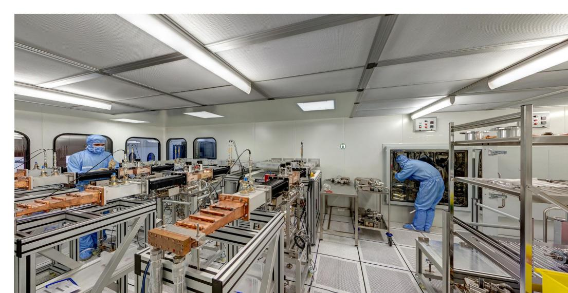
70 m2 ISO5 clean room: Preparation steps and the RF conditioning of couplers, equipped with: ■3 ovens for in-situ backing cycles (up to 200°C), totally automatized, hosting up to 12 couplers. •2 leak test station and a large area for coupler assembly-disassembly.
