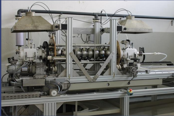
New Electro-Polishing facility dedicated to SC cavities
