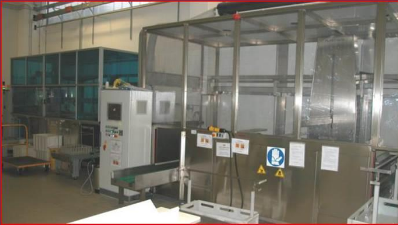
New semi-automatic U.T. cleaning lines and chemical etching lines
