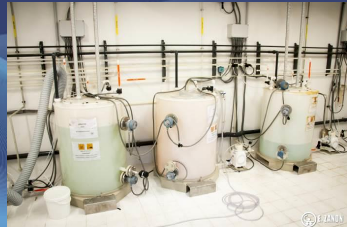
New semi-automatic U.T. cleaning lines and chemical etching lines
